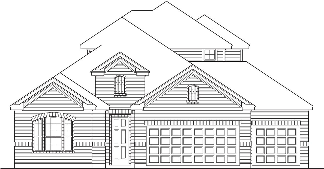
Front Elevation 'A' w/ Optional 2nd Floor, 4' Garage Extension & 3rd Car Garage
